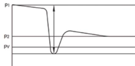
Figure 6: Pressure drop resulting in cavitation [1].
