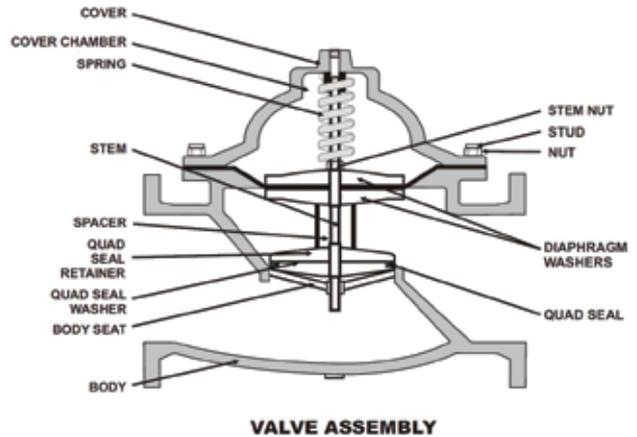
Figure 9b: Proposed valve assembly [2].
