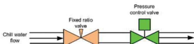
Figure 9a: Proposed valve configuration.
