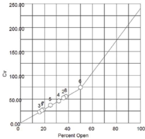
Figure 8: Multi trim valve control curve.
