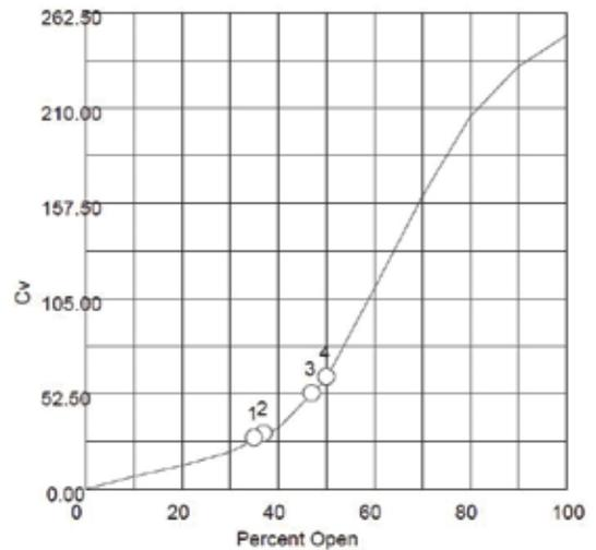
Figure 5: Standard valve control curve.
