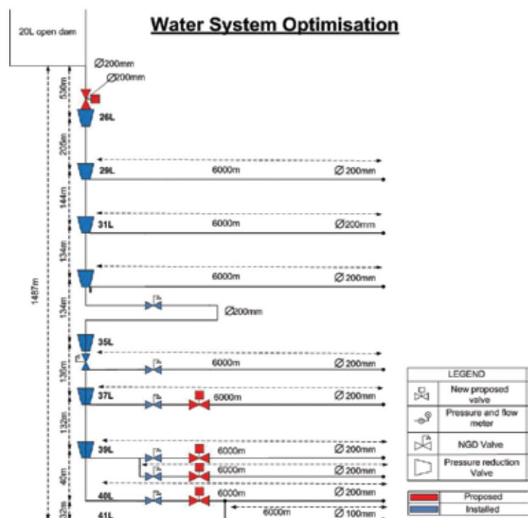
Figure 1: Water reticulation layout.
