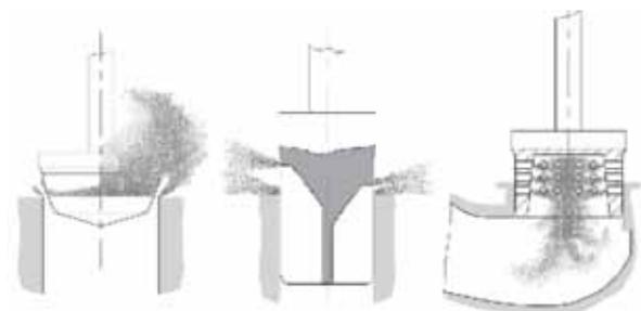
Figure 7: Cavitation limiting trims [1].
