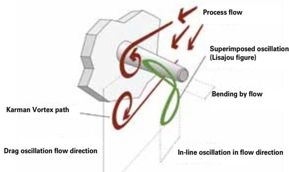
Figure 1: Representation of the oscillation directions.
