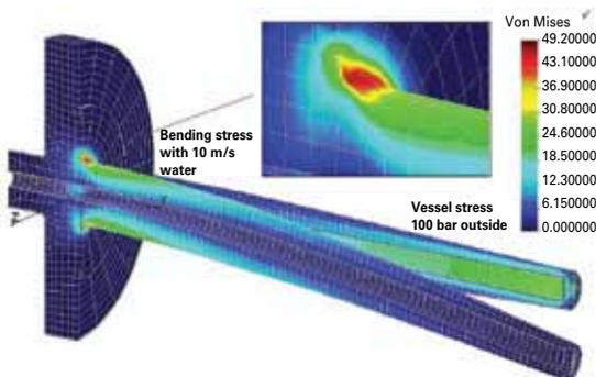
Figure 4: Finite-Element representation with lateral incident flow.
