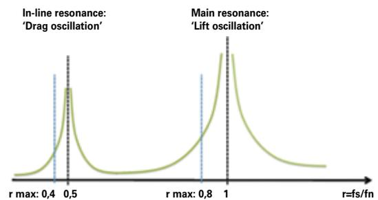
Figure 2: Representation of the in-line and main resonances.
