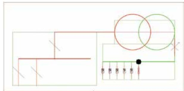
Figure 2: Mini-substation connected network model, allowing for 11 kV cable connections to an 11 kV ring main unit (left), the transformation from 11 kV to 400 V (upper right) and the connection to LV cable circuits at the LV fuses (right).
