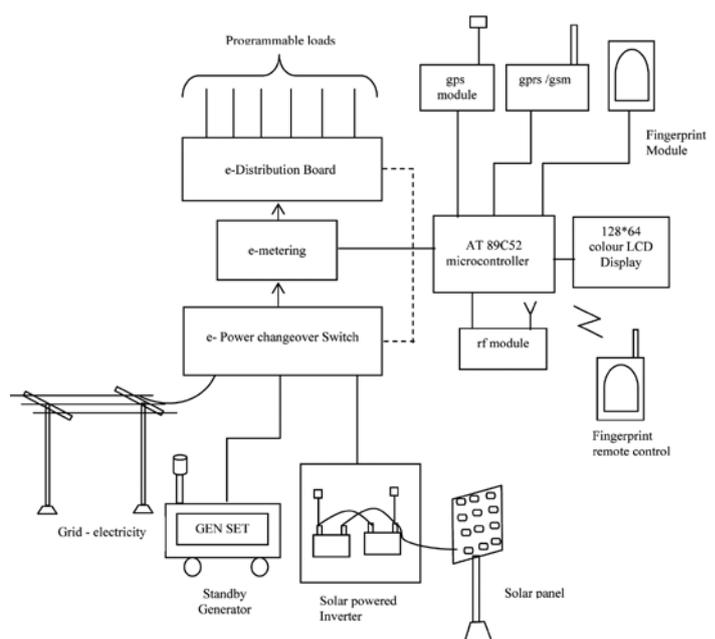
Figure 1: Block diagram of biometric smart distribution board.
