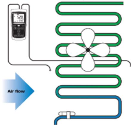
Figure 3: Record evaporator temperature differences as well as min/ max temperatures with a digital thermometer.
