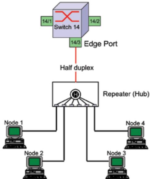
Figure 9.2: Example of edge port operating in a half-duplex mode and connecting to a hub, a collision domain where no other switches are present.
