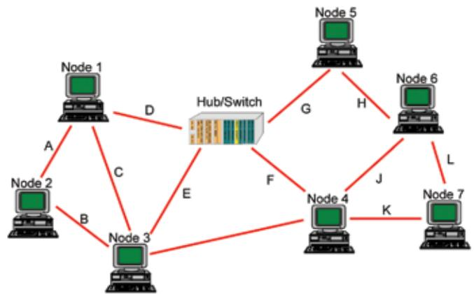
Figure 2.7: In a mesh network, each node is connected to several others and involves the concept of routes – such that a message can take any of several possible paths from source to destination.
