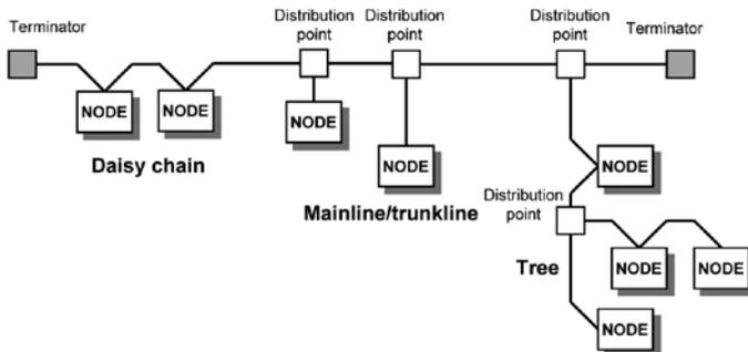
Figure 2.2: Daisy chain, mainline/trunkline and tree configurations.
