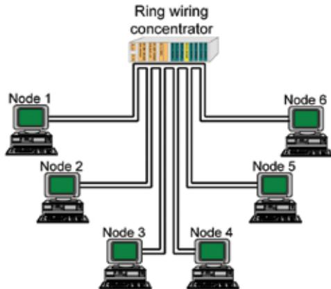
Figure 2.5: Ring network collapsed to look like a physical star.
