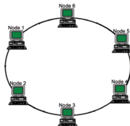
Figure 2.4: In the ring topology, all nodes are connected to a single cable that forms a closed loop or ring, with data flowing in one direction.
