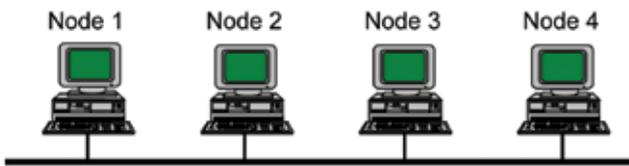
Figure 2.1: In a bus topology all nodes connect to a common media and only one node can transmit at a time.
