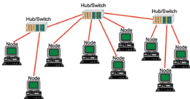
Figure 2.6: A tree topology combines the characteristics of both star and bus topologies.
