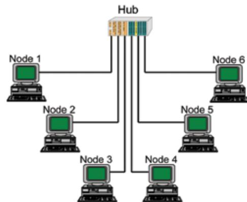
Figure 2.3: In star topology, each node has its own network segment that links it back to a central hub, which controls all communications.
