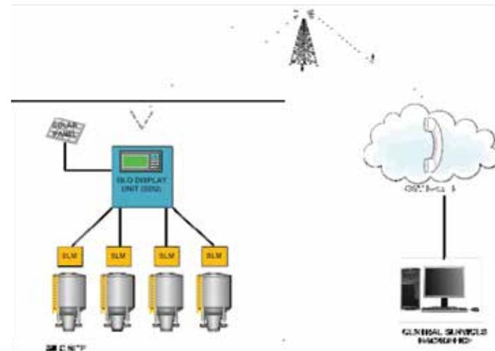
Figure 2: Silo level transmission to control room.
