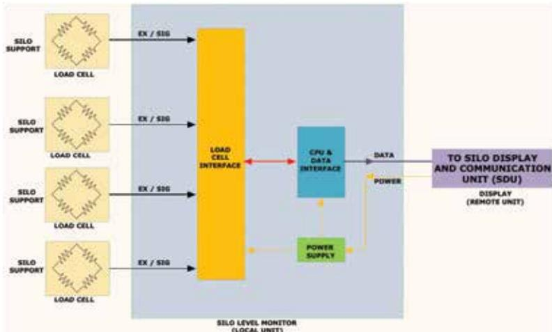
Figure 1: Bulk Explosives level monitoring.
