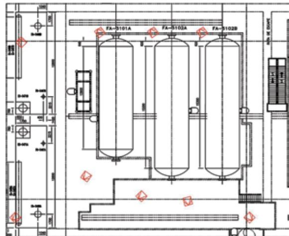
Figure 4: Existing fire detector layout in the area of the production separators.
