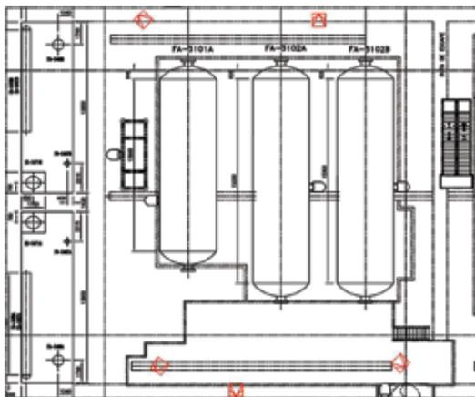
Figure 6: Layout selected because it provided high coverage with a minimal number of detectors.
