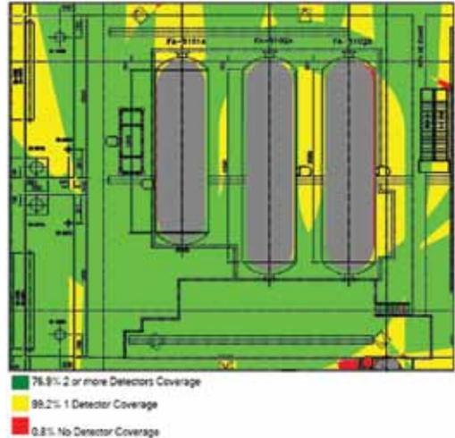
Figure 7: Detector coverage mapping revealed that this design not only reduced the total number of detectors but also improved detector coverage.
