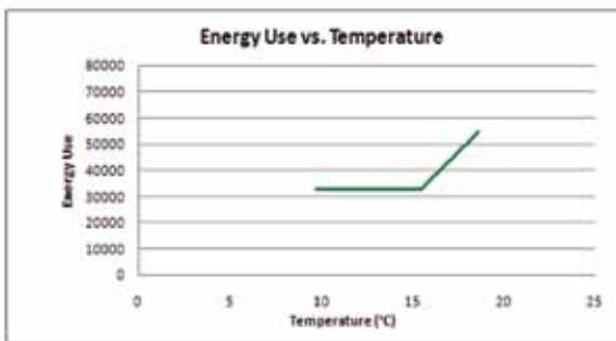
Figure 4: Building behaviour- only cooling done in building.
