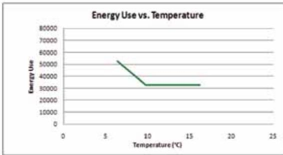
Figure 3: Building behaviour- only heating done in building.
