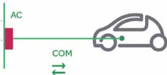
Figure 3: Mode 3 type connection.
