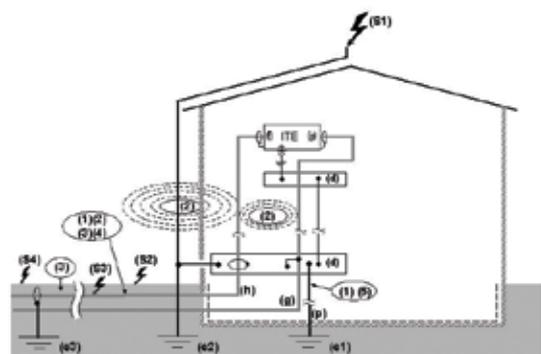
Figure 1: Coupling mechanisms.
