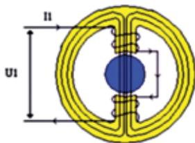
Figure 1: Single phase winding.
