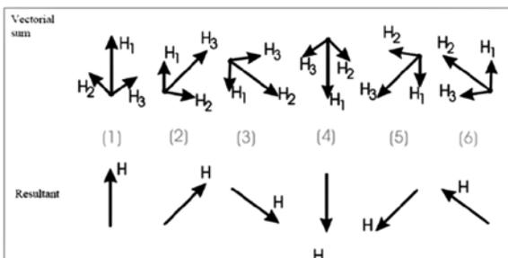
Figure 6: Rotating magnetic field on a three phase motor.
