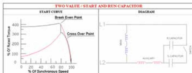
Figure 2: Diagram and starting curve for a single phase motor with start and run capacitors.
