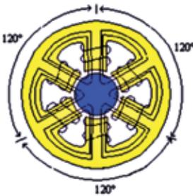
Figure 5: Three phase winding.
