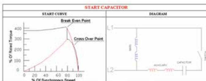
Figure 3: Diagram and starting curve for a single phase motor with start capacitor only.
