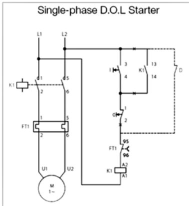
Figure 4: Diagram for a single phase direct on line starter.
