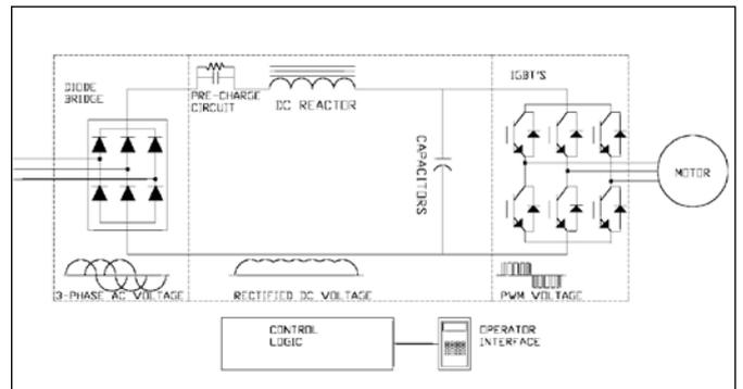
Figure 7: Basic VSD construction.
