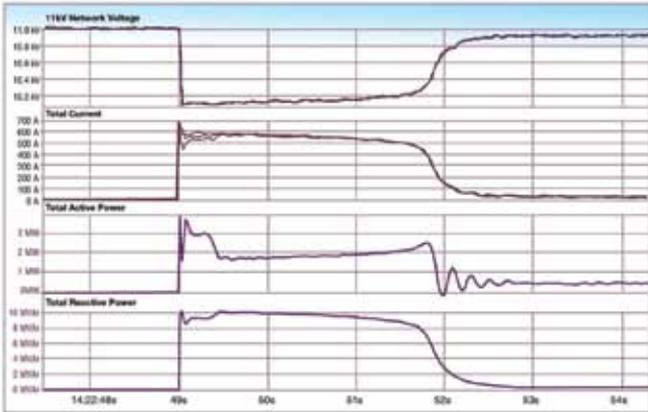
Figure 3: Motor start-up without compensation at 11 kV network voltage.
