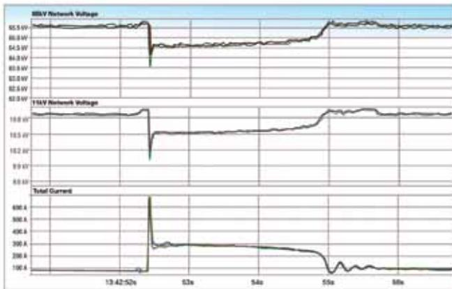
Figure 4: Motor start-up with Elspec EQ-ST only at 11 kV and 66 kV network voltage (66% compensation).
