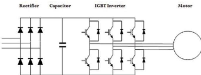
Figure 1: Typical VFD unit configuration.
