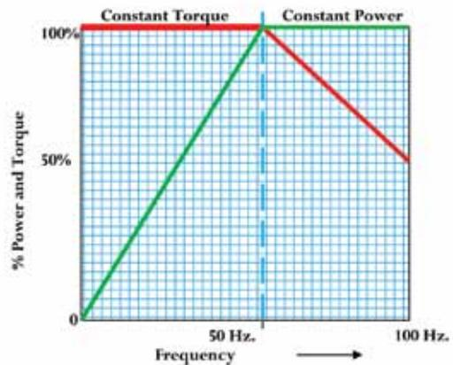
Figure 3: Typical torque power curve for a VFD.
