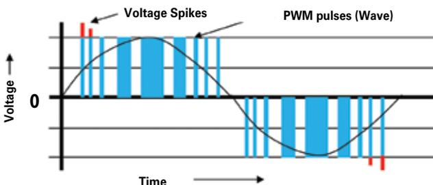
Figure 2: Pulse Width Modulation Wave.
