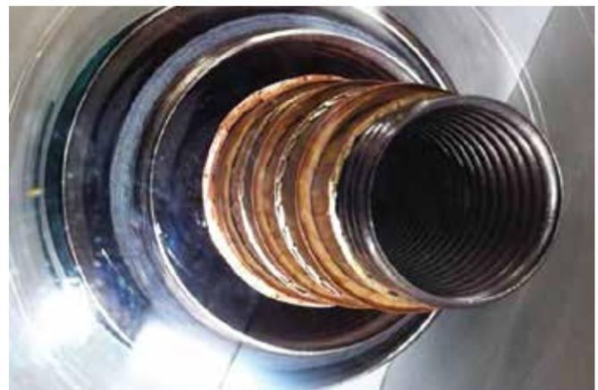
A typical HTS cable. The three concentric conductor layers are barely visible, yet each can handle almost 2 000 A.
