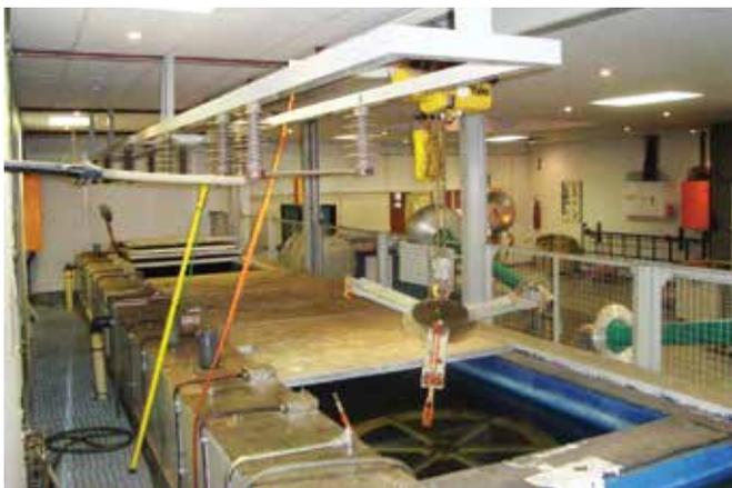
*An accelerated ageing facility for testing MV XLPE cable.*
