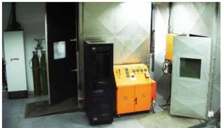
*A fire performance test facility, with a flame propagation chamber on the left and a smoke emission chamber on the right.*
