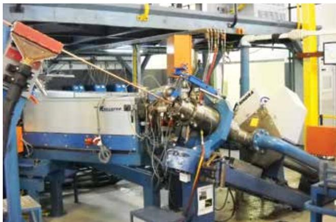
A modern MV and HV triple head XLPE extruder.
