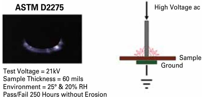
Figure 2: Cylindrical electrode test.
