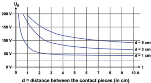
Figure 5: Arc-burning voltage between the contact pieces of switching devices at standard temperature and pressure.
